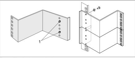
Figure 6: Mounting the support brackets
